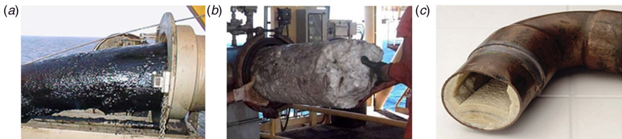
Fig. 1 Solid deposits due to (a) wax plug [15], (b) hydrate plug [31], and (c) \text{CaCO}_3 scale [32]
