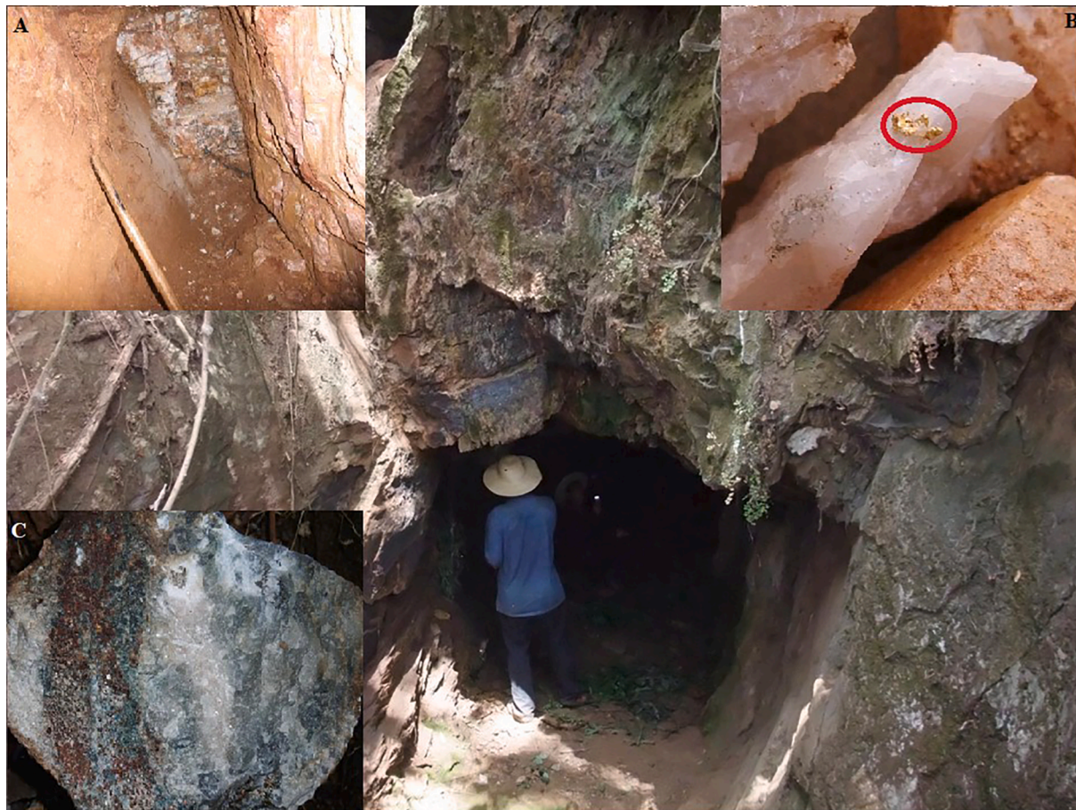
Fig. 12. Adit for exploration minerals, (A) Gold-bearing quartz vein, (B) Visible gold in quartz vein, (C) Ore deposit contains pyrite and chalcopyrite.
