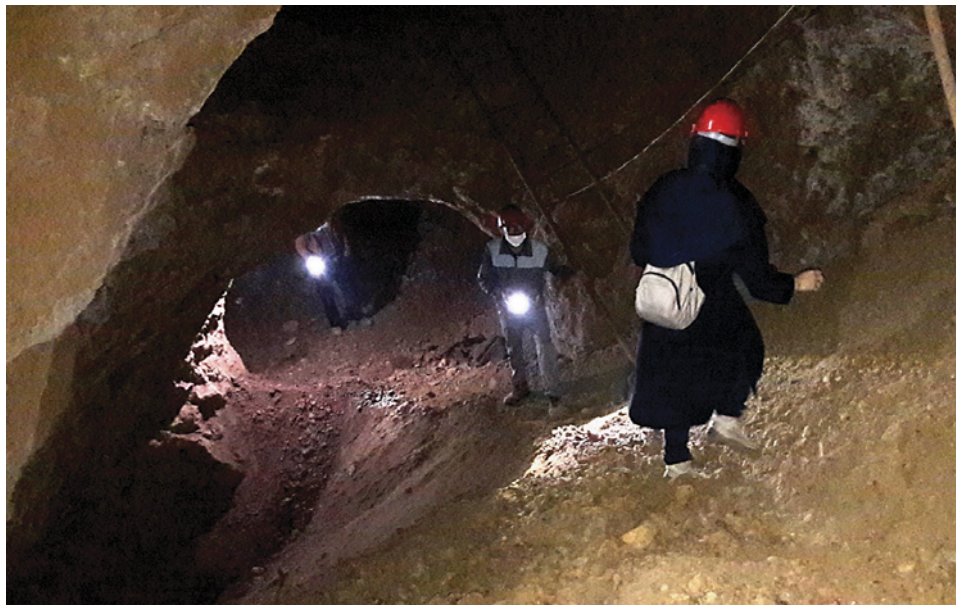
Figure 15. An old stope that has been back-filled to create a path for miners. Photo by R. Shirdam.
