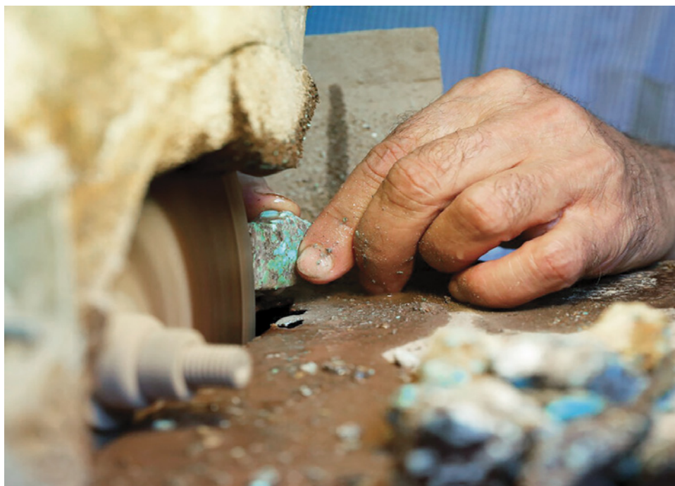
Figure 27. Slabbing rough turquoise in a lapidary workshop in Mashhad. Photo by M. Bakhshandeh.
