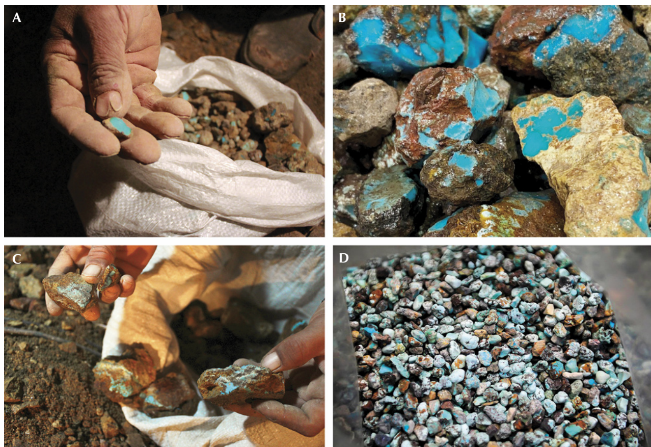
Figure 25. The four major quality levels of rough turquoise production from Neyshabur: turquoise nuggets (A), turquoise with the host rock attached (B), chalky turquoise (C), and turquoise chips (D). Photos by B. Shirdam.
