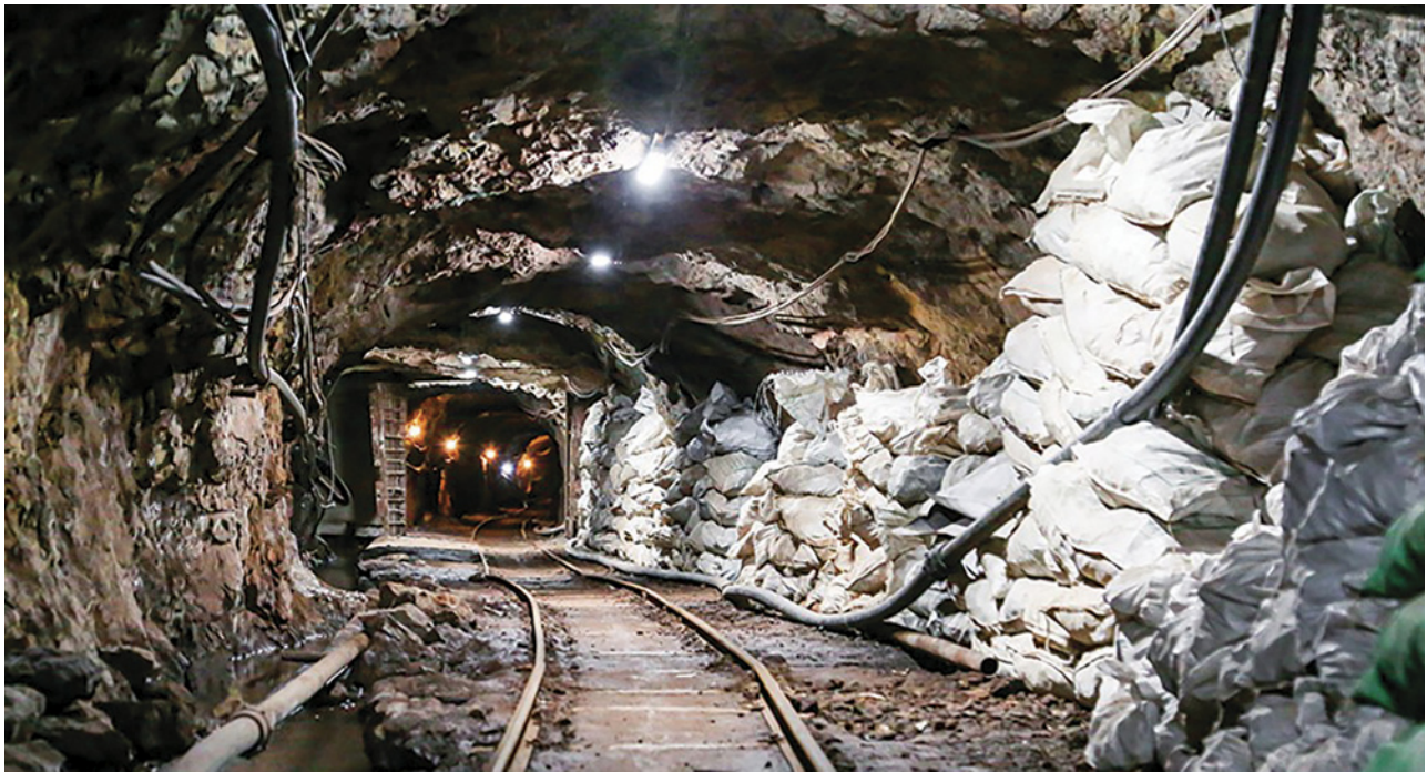
Figure 22. Compressed air tubes in the tunnels. Photo by R. Azizi.
