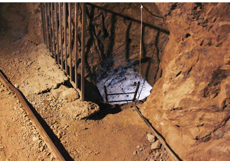
Figure 16. The winze to the lower Zahk tunnel. Photo by B. Shirdam.
