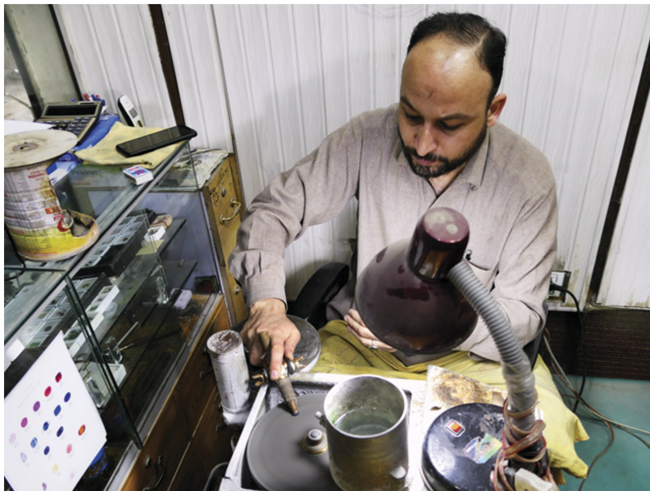
Figure 11. A highly experienced cutter, Mr. Sajid, guided the authors through the entire process of faceting with the angoora . Photo by Shakeel Anwar Khan.
